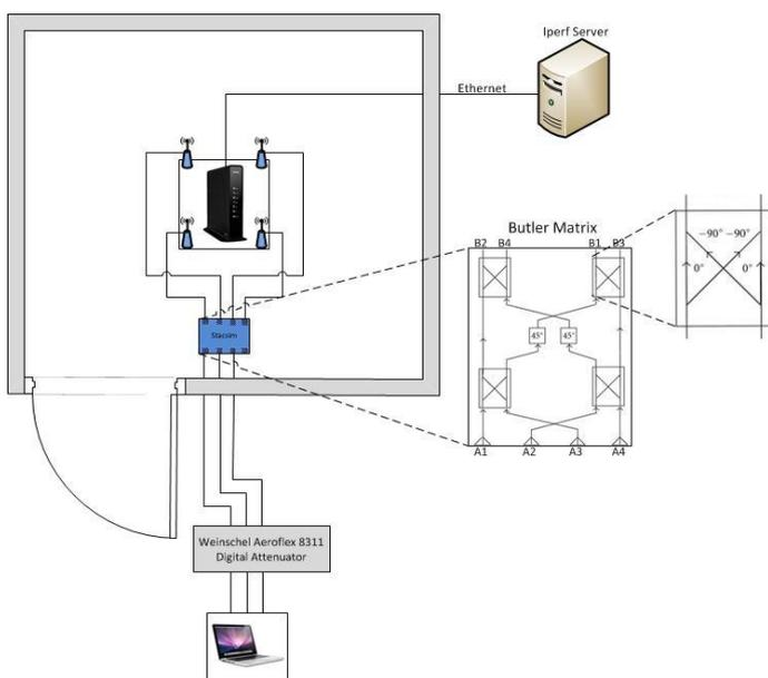
Allion leverages a unique solution that combines a large anechoic chamber (3m x 3m x 3.5m) coupled with inline programmable attenuation and butler matrix used to simulate the multi-path that is usually seen in an over-the-air environment.
