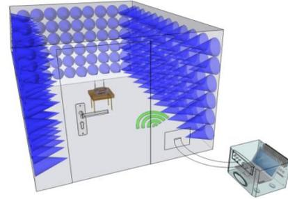
Throughput performance is base-lined by collecting throughput measurements based on the changing RF conditions (channel fading) by performing a throughput speed test at each attenuation level – incrementally increasing the attenuation between the station and wireless gateway.
