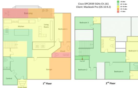
The results above support the results reported from the Rate vs. Range testing that using a gateway that leverages both the benefits of 802.11n and more advanced hardware (3x3 antenna configuration) also results in overall better coverage as compared to either legacy 802.11a/b/g or lesser 802.11n technologies.
