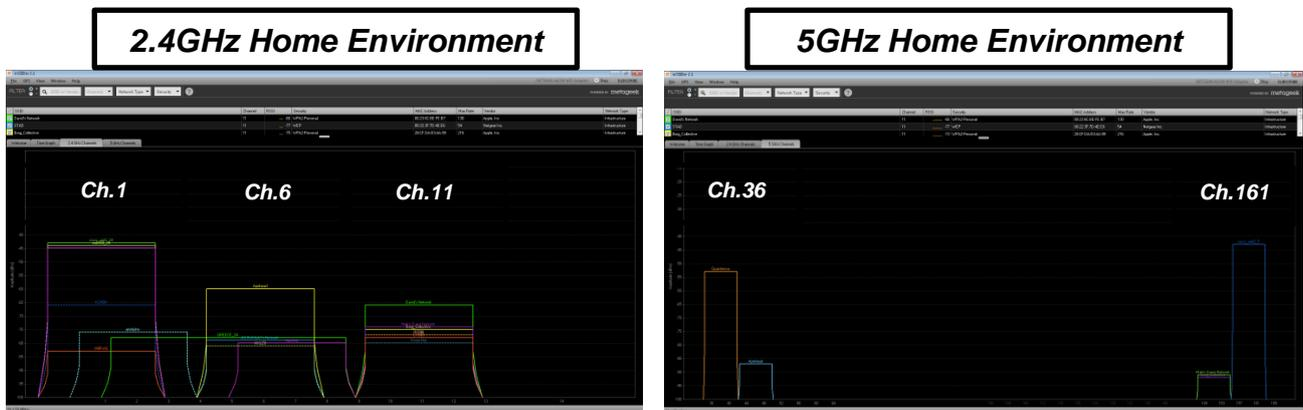
The image above shows that the 2.4GHz band not only has several APs across the entire spectrum, but a noticeable amount of RF noise generated due to the limited channels. On the other hand, the 5GHz band shows plenty of non-overlapping channels. The extra channels helps prevent RF interference, which results in a better end-user experience.
